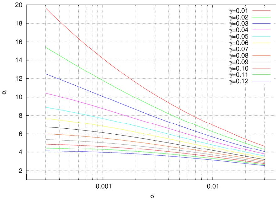
Fig. 5. Nomogram (Cieplik, 2009a) for the determination of maximal amplitudes at the free coasting of the symmetric machine and of the machine of a linear vibration trajectory.
