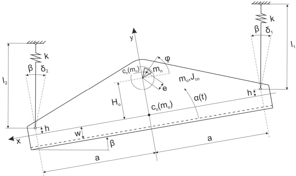
Fig. 1. Schematic presentation of the suspended screen
